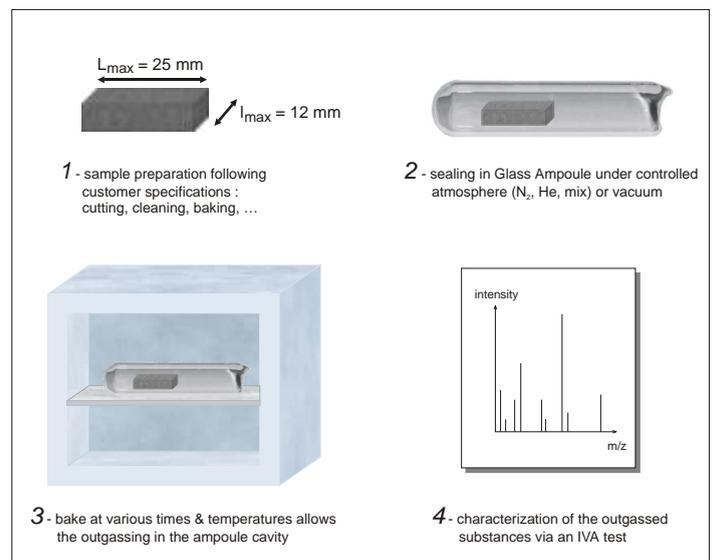
The Material Outgassing Characterization test was initially developed to assist the microelectronic and optoelectronic component manufacturers. Its broad scope of application, however, makes it a powerful tool to address the needs of a larger community.
